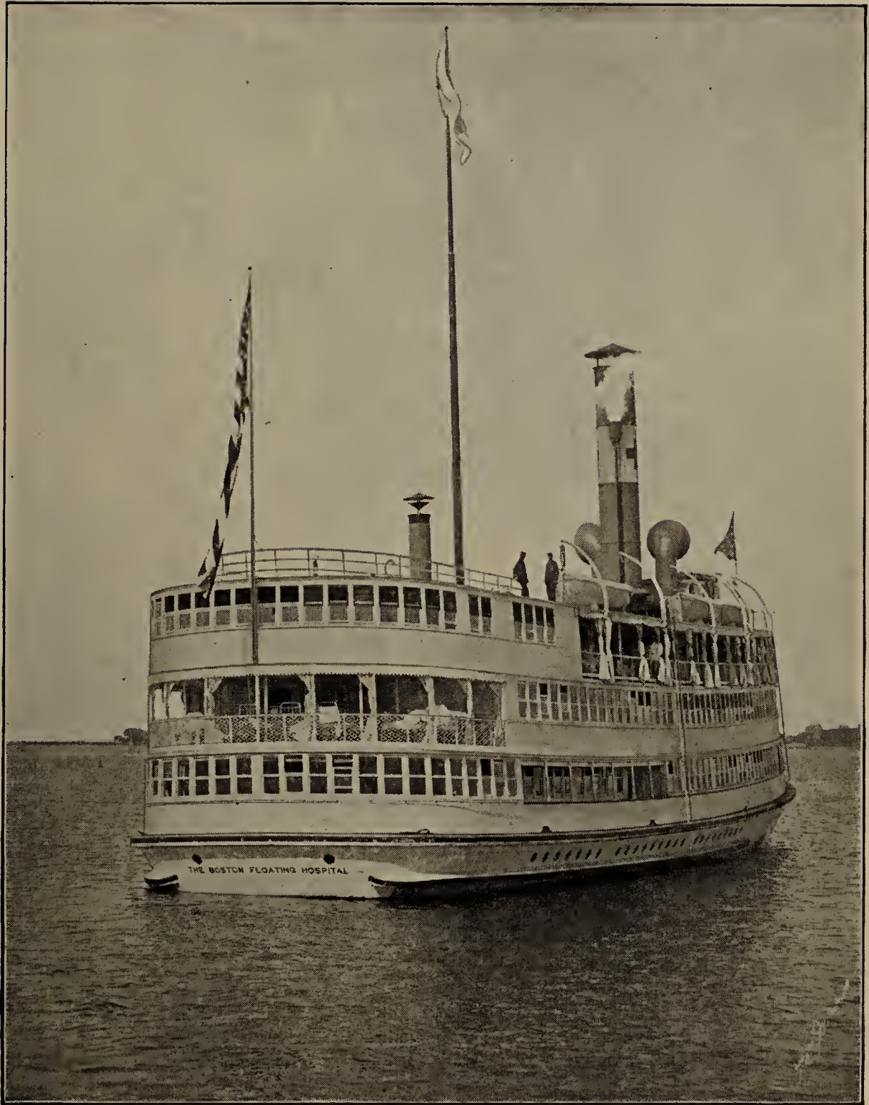
STERN VIEW, SHOWING THE OPEN-AIR PERMANENT WARD
